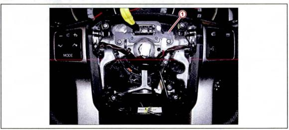
Steering Wheel Switch Wire Harness Retainer Bracket
