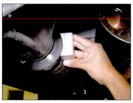
Figure 13. INCORRECT Placement of Protractor
