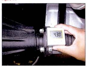
C. Obtain the Propeller Shaft to Pinion Joint Angle (J/A).
