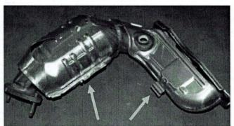
Catalytic converter and exhaust manifold heat shields
