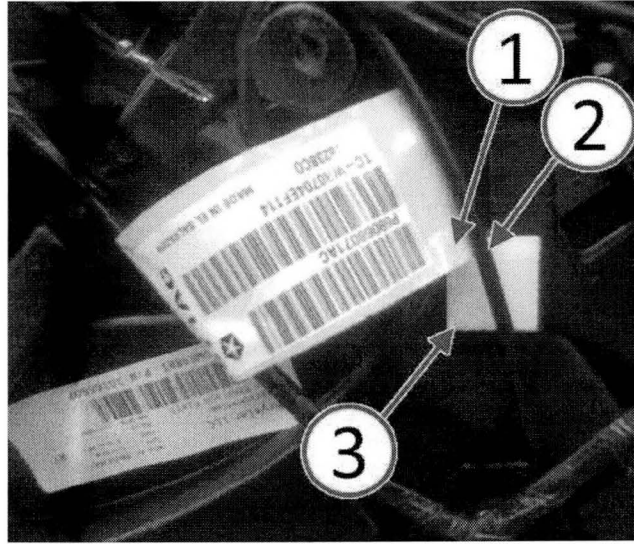
Fig. 11 Dual Lock Interference Conditions
