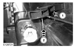
5. Fold the protruding ends of the split / cotter pin.
