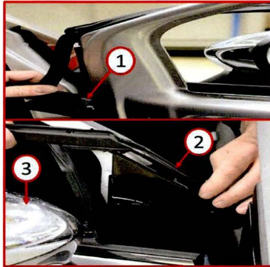
Fig. 4 Glass Run Weatherstrip Removal
