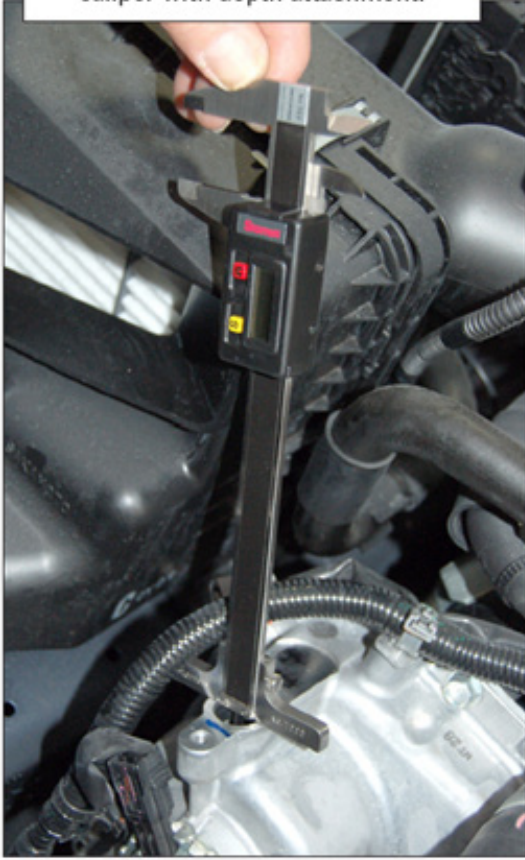
Measurement taken using digital caliper with depth attachment.
