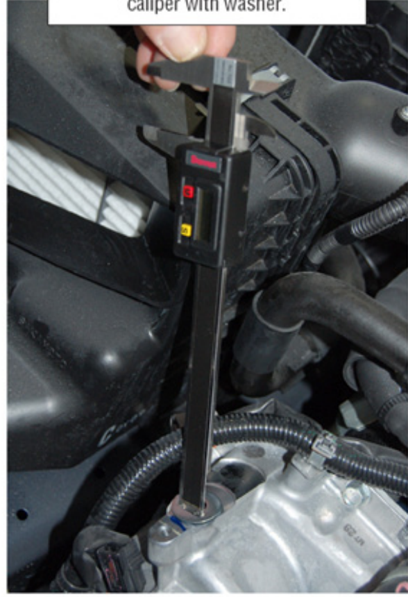
Measurement taken using digital caliper with washer.
