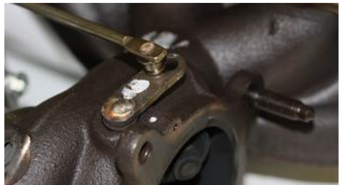
Figure 1. Disconnected wastegate linkage.
