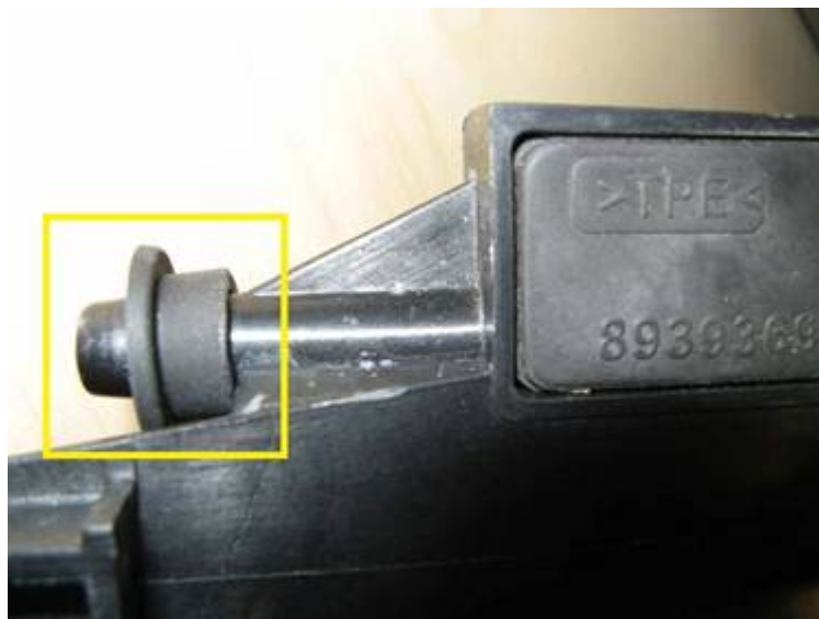
Figure 5. Ring seal installed on headlamp air tube.
