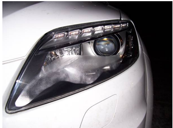
Figure 1. Moisture in headlamp.
