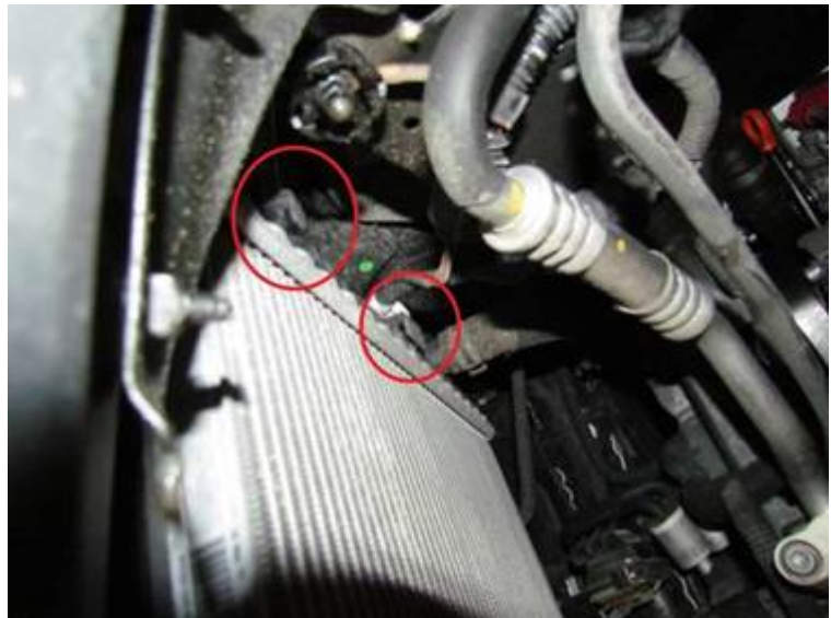
Figure 8. Upper exit air duct attachment points to additional radiator.
