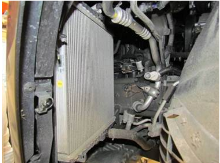
Figure 6. View of additional radiator with wheel well liner removed.
