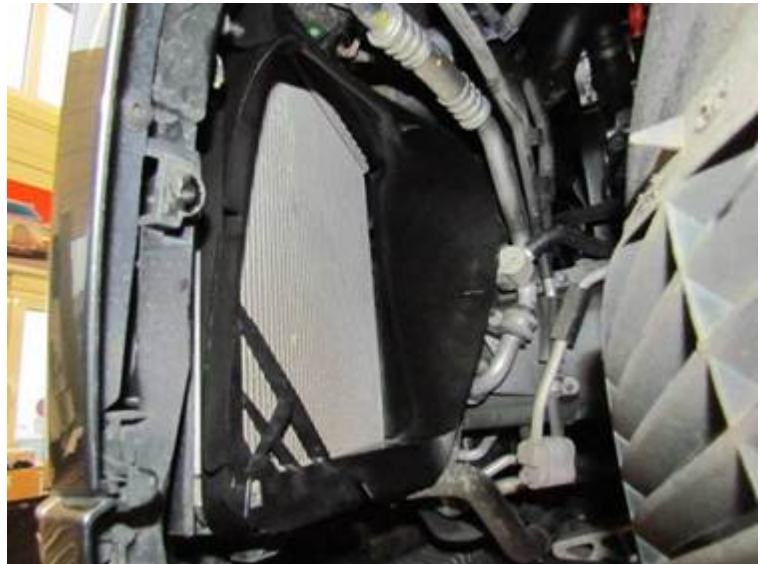
Figure 9. Exit air duct installed.
