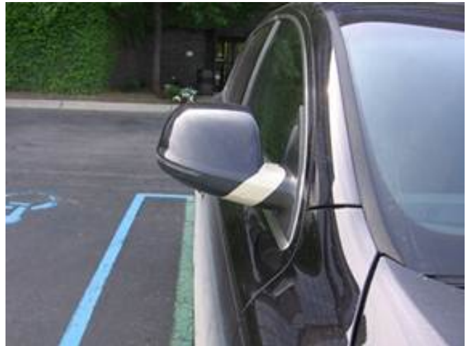
Figure 1. Tape applied to rotation collar seam.
