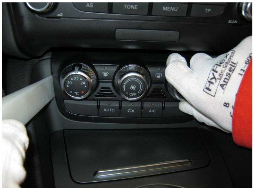
Figure 4. Removing the Climatronic Control Module.
