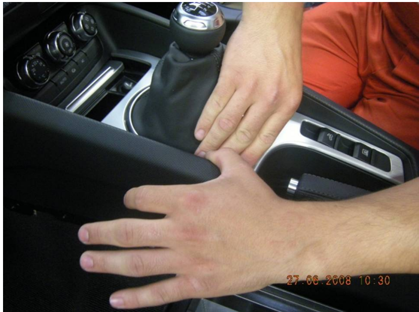
Figure 9. Pressing in the left center portion of the console trim.
