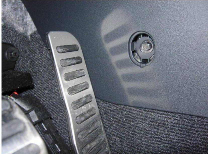
Figure 2. Mounting bolts for the console side trim.
