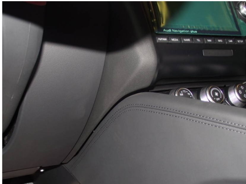
Figure 7. Gap achieved between the upper and lower sections of the center console after adjustment.
