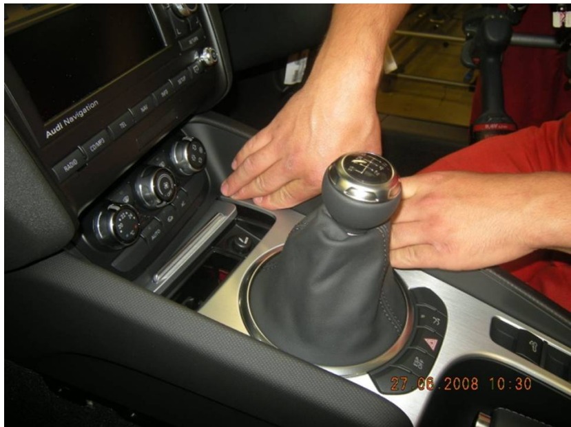
Figure 10. Pressing the right side of the console trim into place.
