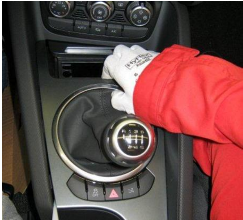
Figure 3. Removing the center console trim.
