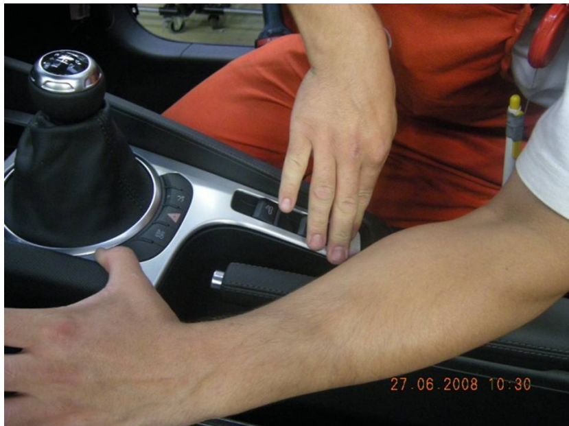
Figure 8. Installation of the center console trim.
