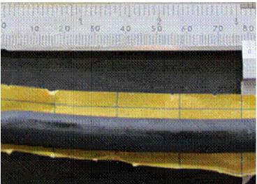
Figure 3. Butyl cord sealant, 10mm diameter.
