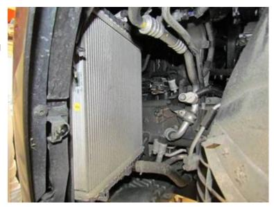
Figure 8. View of charge air cooler with wheel well liner removed
