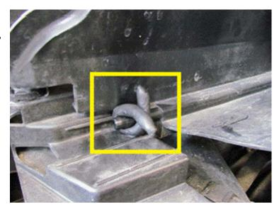
Figure 5. Initial butyl cord shown on guide tube.
