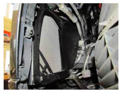
Figure 11. Charge air cooler exit air duct installed.
