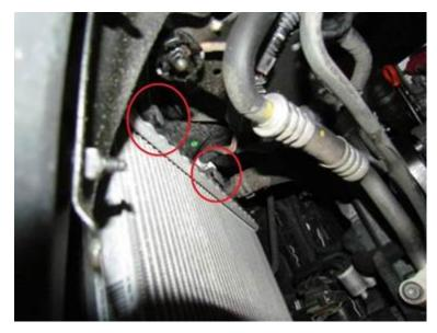
Figure 10. Upper exit air duct attachment points to charge air cooler.
