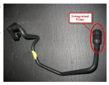
Figure 2. Updated ventilation hose with integrated filter.
