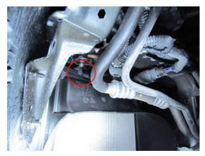
Figure 12. View of exit air duct affixed to mounting hook.
