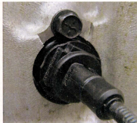
New sensor installed without retaining clip
