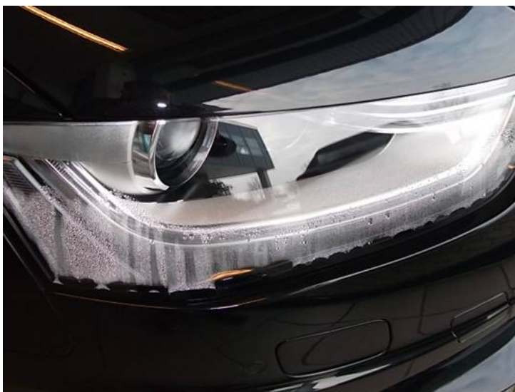
Figure 1. Xenon headlight with a significant amount of water collecting at the base of the lens.
