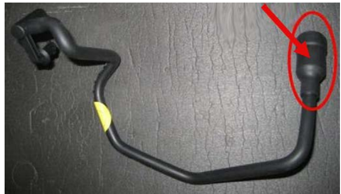
Figure 2. Updated ventilation hose with integrated filter.
