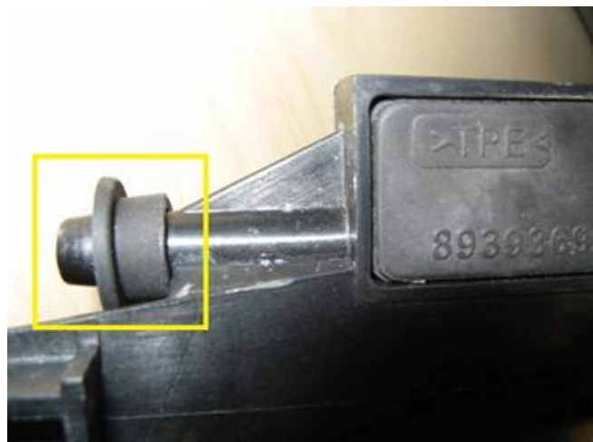
Figure 5. Ring seal installed on headlamp air tube.
