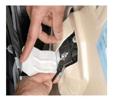
1. Disengage the door trim, without detaching the inside door handle cable. DO NOT LET THE TRIM PAD HANG FROM THE HANDLE CABLE OR THE WIRE HARNESS.
