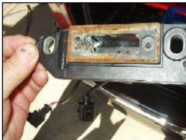
Figure 2 – Corrosion around License Plate Light
