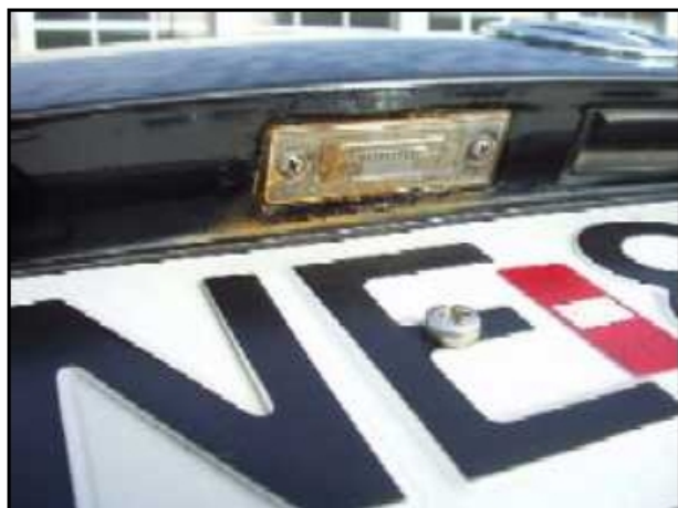
Figure 1 – Corrosion around License Plate Light
