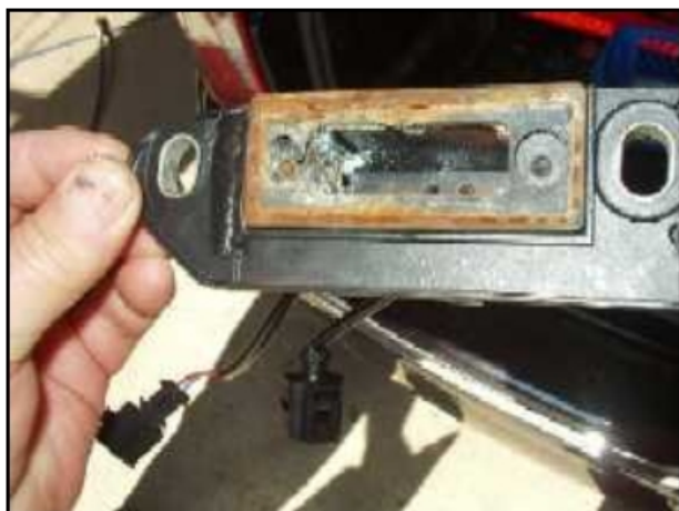
Figure 2 – Corrosion around License Plate Light
