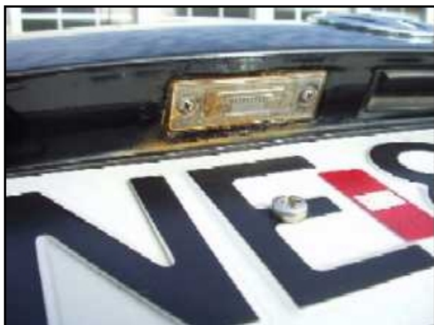
Figure 1 – Corrosion around License Plate Light
