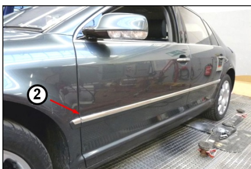
Figure 2 – Central protective strip
