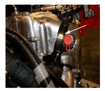
9. After alignment of all the joints, install and tighten a new clamp at the turbocharger (if removed earlier).
