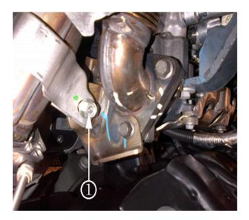
12. Install the mounting bolt (1). If the mounting bracket was removed, align and install the bracket. If the bolt will not line up, bend or shim the bracket until alignment is possible.
