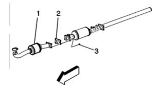
5. Loose or disconnect the four flange mid-joint bolts located after the catalytic converter.
