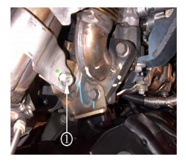
3. If the joint has a gap on either the left or right side, loosen or remove the turbo exhaust pipe mounting bolt (1) as shown in the illustration above.
