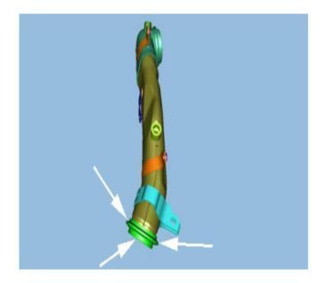
**Note:** The illustration above is the updated turbocharger exhaust pipe with a pilot flange.
