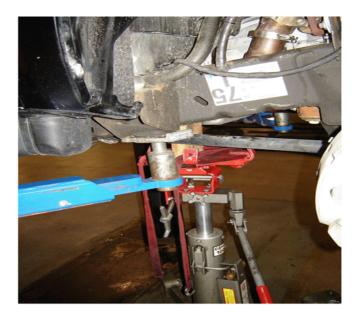
7. Using a transmission jack, align the exhaust pipe, downpipe and the turbocharger exhaust pipe flanges until all mounting joints and the flanges are flush and parallel with no or minimal load or force applied. This could include adjusting the mounts as necessary, allowing the flanges to sit flush with the exhaust in a neutral state, using care not to compromise clearances around the exhaust.
