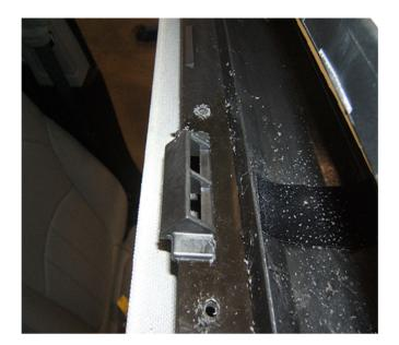
Important: When drilling holes, be careful not to drill through the headliner.
