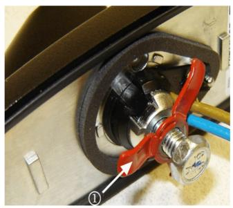
Though difficult to detect evidence of impact damage, upon inspection of the antennas returned in warranty, there is a likelihood this damage occurred during vehicle transportation to dealerships. The result of impact damage is most often to the underside retainer (1), which is found to be bent backward or otherwise damaged and no longer provides proper retention.
