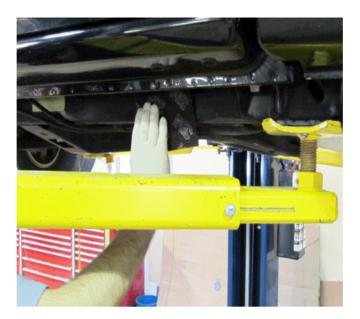
6. Remove any residual wax, oil or rust by wiping the frame down with a Scotch-Brite<sup>™</sup> pad and wax/grease remover.
