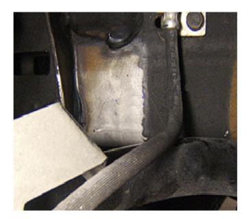
4. Using a rag and wax/grease removing solvent, remove the wax coating from the truck frame in the designated repair area. The graphic above shows an example of a small portion of the wax coating removed.
