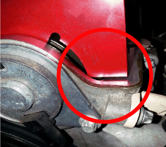
Front Cylinder Head with Tool Showing Exciter Wheel Misalignment
