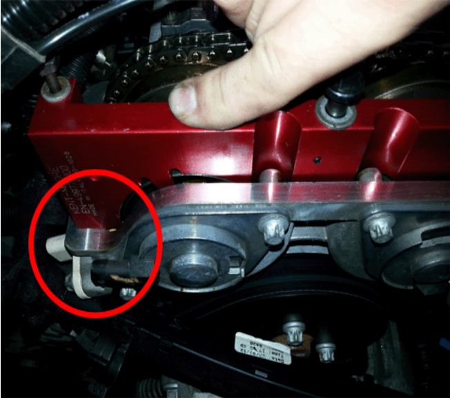
Rear Cylinder Head with Tool Showing Proper Exciter Wheel Alignment
