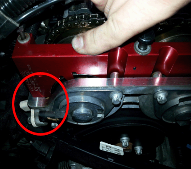
Rear Cylinder Head with Tool Showing Proper Exciter Wheel Alignment
