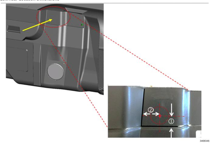
**Important:** To better control the accuracy of the rear locations, it is critical to mark the location of the horizontal line first. Measure the distance upward (1) in several areas, and using a marker or tape, position a line at that level. Then, along that line, mark the intersecting point for the second measurement (2).
