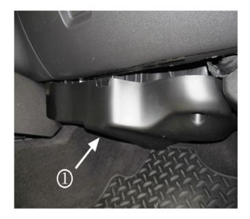
1. Remove the instrument panel insulator (1). Refer to Instrument Panel Insulator Replacement in SI.
