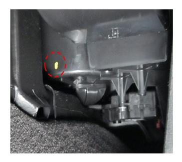
4. Note the position of the lower HVAC case and mark a location to drill a hole in the case on the rounded corner facing the driver footwell area. The mark should be approximately 13 mm (0.50 in) upward from the bottom surface of the case.
