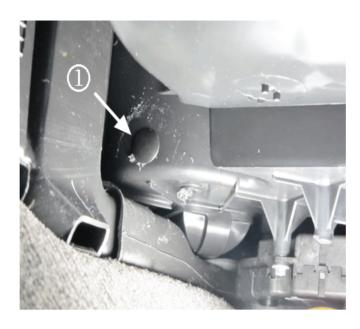
**Important:** To improve sealing of the plugged hole, apply a small amount of RTV, GM P/N 12378521 (in Canada, P/N 88901148), or equivalent, to the push pin prior to installation.
