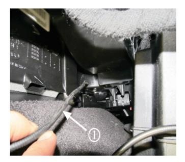
6. Insert the borescope (1) and look to see the position of the horizontal belt seal around the heater core.
