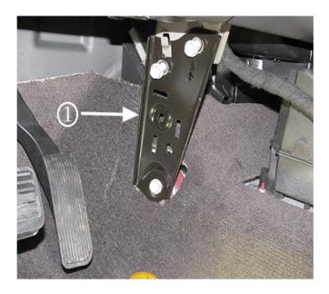
3. Remove the instrument panel lower brace bezel and center support bracket (1). Refer to Instrument Panel Center Support Bracket Replacement in SI.
