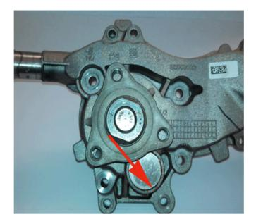
Slight coolant staining around the perimeter of the cover plate.
