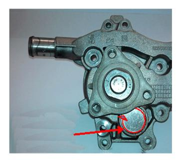
3. Apply a small bead of RTV Engine Sealant, P/N 88861417 (in Canada, P/N 88861418) to the seam around the perimeter of the reservoir cup plug.
