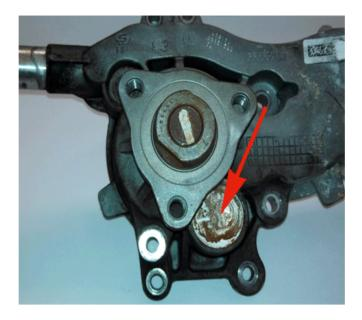
Significant coolant residue on the cover plate.
