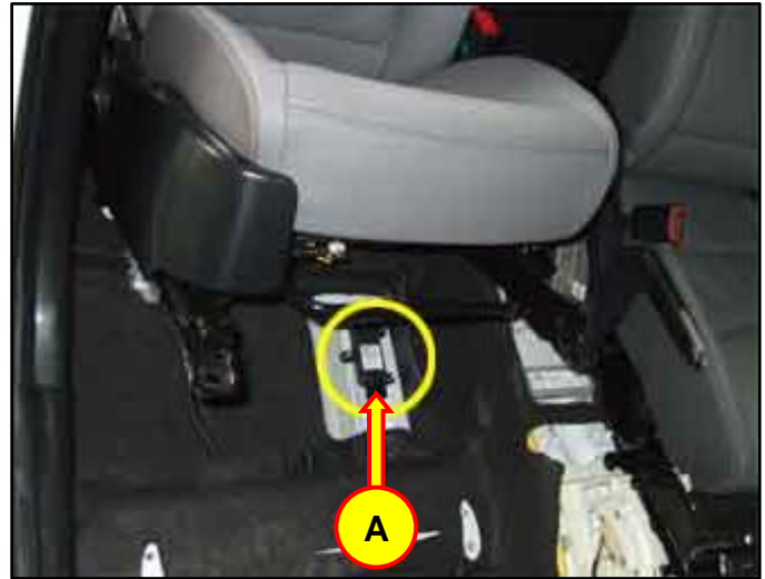
Yaw Rate/"G" Sensor tightening torque: 3.9 ~ 5.9 N.m (0.4 ~ 0.6 kgf.m, 2.9 ~ 4.3 ft-lb, 34.8 ~ 51.6 in-lb)
