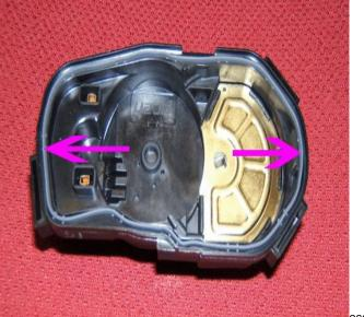
14. Verify that the TP sensor cover gasket is secure and properly positioned.
