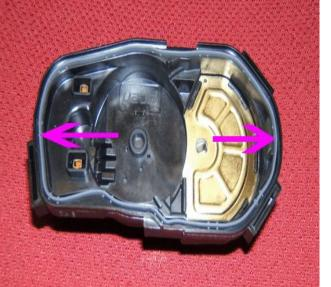
10. Verify that the TP sensor cover gasket HAS REMAINED in the TP sensor cover as shown. Ensure that the gasket is accounted for and remains with the old TP sensor cover.
