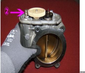
**Note:** If one or both of the TP sensor cover female throttle actuator motor terminals (1) HAVE BEEN retained on the throttle actuator motor male terminals (2), remove and discard those female terminals.
