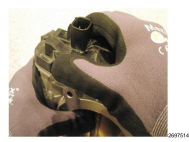
8. Hold the throttle body with your hand, so that the TP sensor cover is facing upward. Grasp the TP sensor cover and carefully lift it up and separate it from the throttle body.
