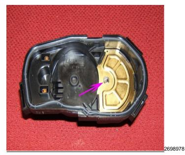
**Note:** If the TP sensor drive slot orientation is not aligned as shown, use a small flathead screwdriver to gently rotate the TP sensor drive slot clockwise to the wide open throttle (WOT) position as shown.
