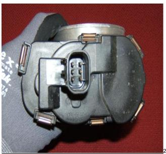
**Note:** DO NOT mount the throttle body in a vise. The throttle body can be set on the top of a soft protected workbench area.
