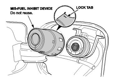
• Pilot: Pull the mis-fuel inhibit device off the filler neck and toward the rear of the vehicle.
