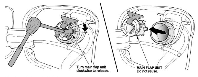
8. Turn the main flap unit clockwise until it stops, then remove it.
