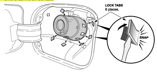
• *Pilot*: Break the four lock tabs then turn the mis-fuel inhibit device clockwise.
