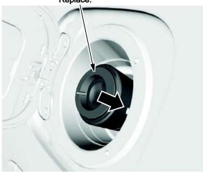
4. Set the capless wrench and slightly turn the main flap unit counterclockwise. NOTE: The main flap unit may only move a small amount. This is normal.
