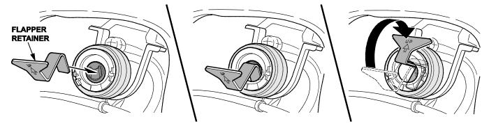
6. Insert the capless pick under the lock tab and release the lock by turning the pick counterclockwise.
