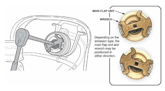
5. Remove the capless wrench and install the flapper retainer onto the main flap unit as shown to keep the flap open.
