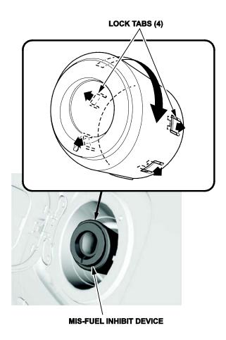
3. Remove the mis-fuel inhibit device.
