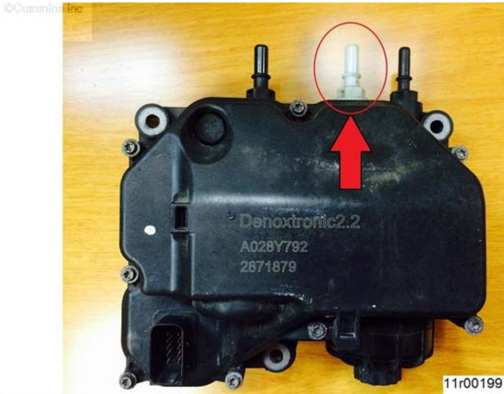
Figure 1, Revised Backflow Connector, Part Number 4387302, Installed in the Aftertreatment DEF Dosing Unit
