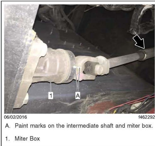
Fig. 7, 90-Degree Miter Box and Intermediate Shaft
