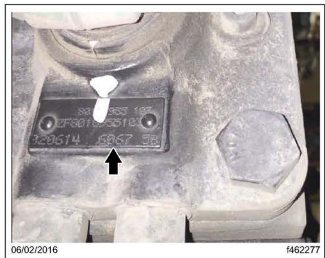
Fig. 2, Steering Gear Type Plate, Four-Digit Serial Number
