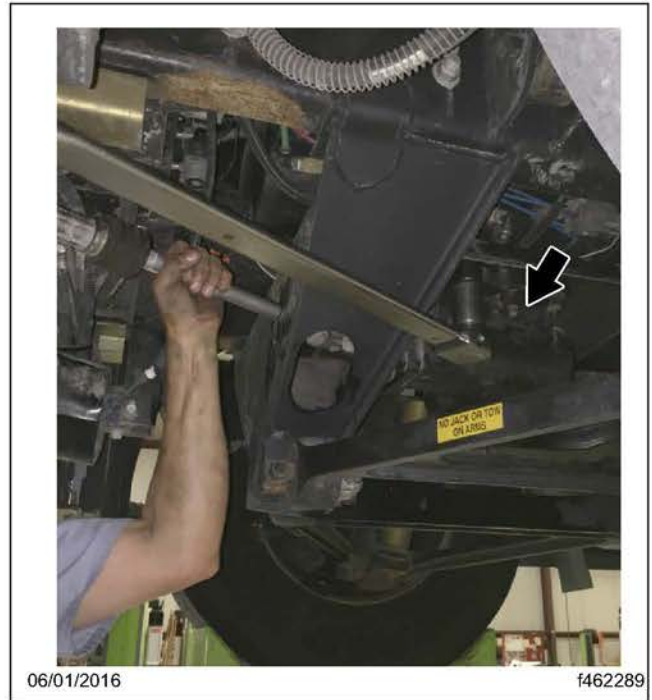
Fig. 15, Positioning the Steering Gear (box is hidden by the A-frame)
