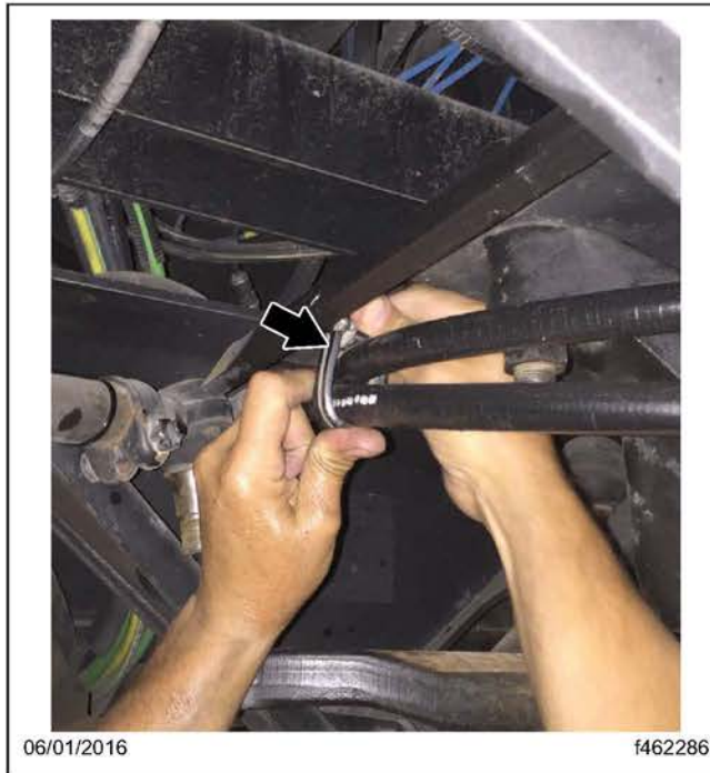
Fig. 16, Mounting the Hydraulic Hoses to the Frame
