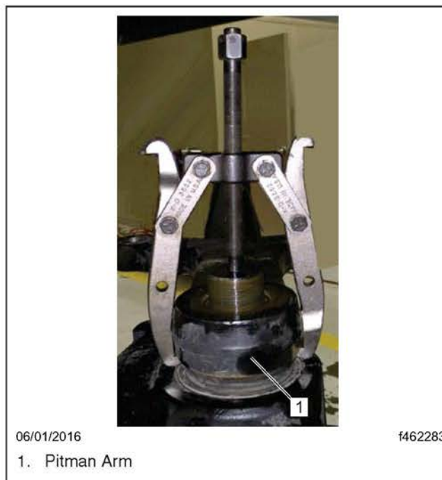
Fig. 11, Removing the Pitman Arm with a Two-Arm Puller
