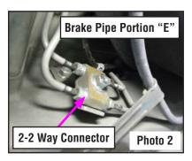
**IMPORTANT:** Even if the 2-2 Way Connector appears to have been previously rust-proofed, the balance of this recall procedure must still be completed in its entirety.
