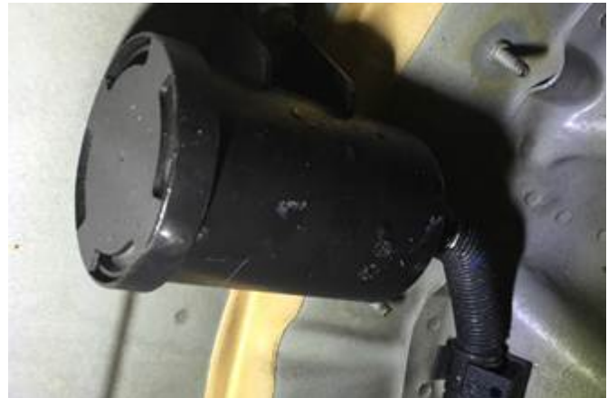
Figure 1. Ventilation tube of the activated charcoal filter.
