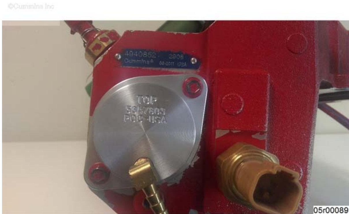
Figure 2, New Low Pressure Regulator Fuel Control Cover, Installed on ISL G CM2180 EJ Low Pressure Housing
