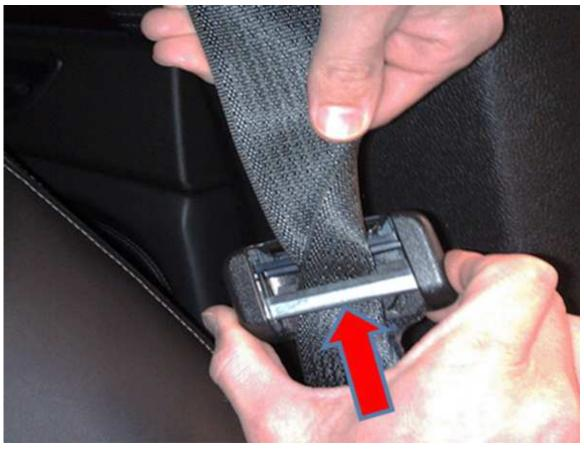
2. Grasp the latch plate and push the plate upward over the fold until the twist is removed.
