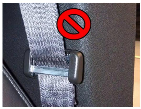
As shown in the graphic above, some customers may comment that the driver or passenger side seat belt is twisted or the latch plate is facing backward on the webbing. Note that the tip of the latch plate is **incorrectly** positioned outboard of the webbing when stowed.
