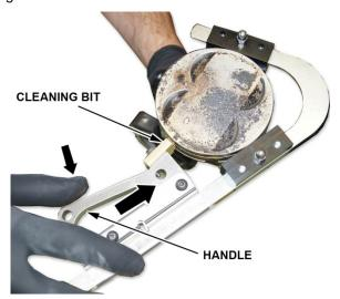
5. Once the cleaning bit is in the appropriate ring grooves of the piston, make sure the tool handle clicks in to place. NOTE: There is only one notch on the tool for the handle to engage.
