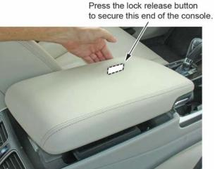
5. Press the lower lock release lever until it clicks into place.
