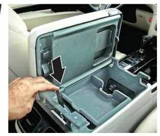
2. Press the upper lock release lever to release this end of the lid.
