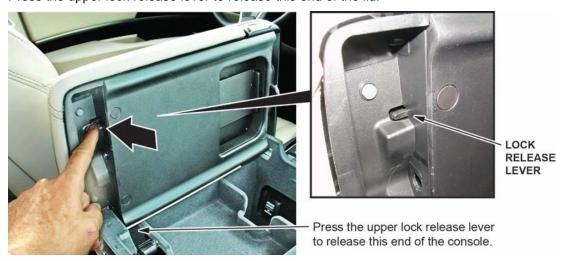
3. Press the lock release button to release the lid, then remove it.
