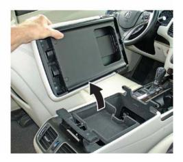
4. Install the new center console lid to the center console as shown, then press the lock release button and maneuver the lid until it clicks into the hole to secure it into place.
