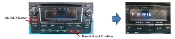
• **IMPORTANT**: Do not remove the USB or turn the ignition off while software is updating. The updating procedure will take approximately 8 minutes to complete.
