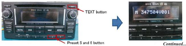
With the version ID displayed, press the CD/AUX button along with station preset buttons
