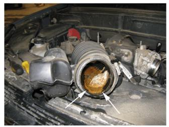
Technicians may find the presence of DTCs P0101, P0171, P0172, P0174, P0175, P1516, P2177, P2178, P2179, P2180, P2187, P2188, P2189, and/or P2190 along with either ice or oil deposits in the air inlet duct.
