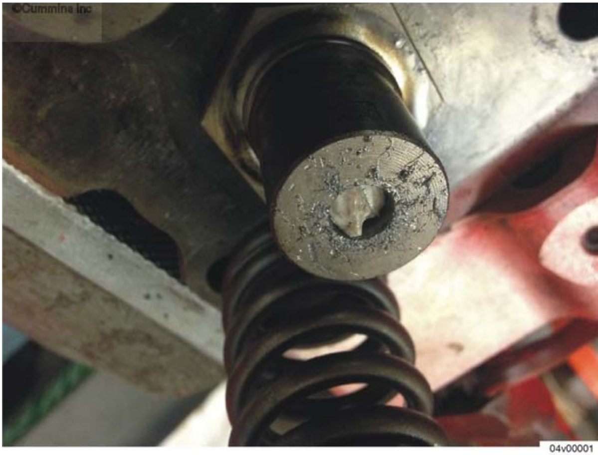
Figure 1: Fractured Fuel Pump Ceramic Pumping Plunger
