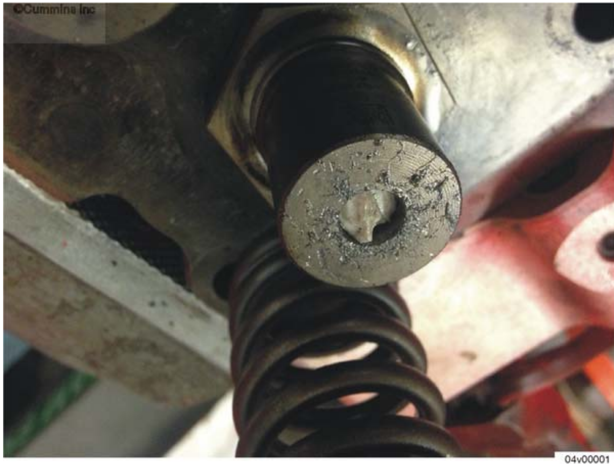
Figure 1, Fractured Fuel Pump Ceramic Pumping Plunger.
