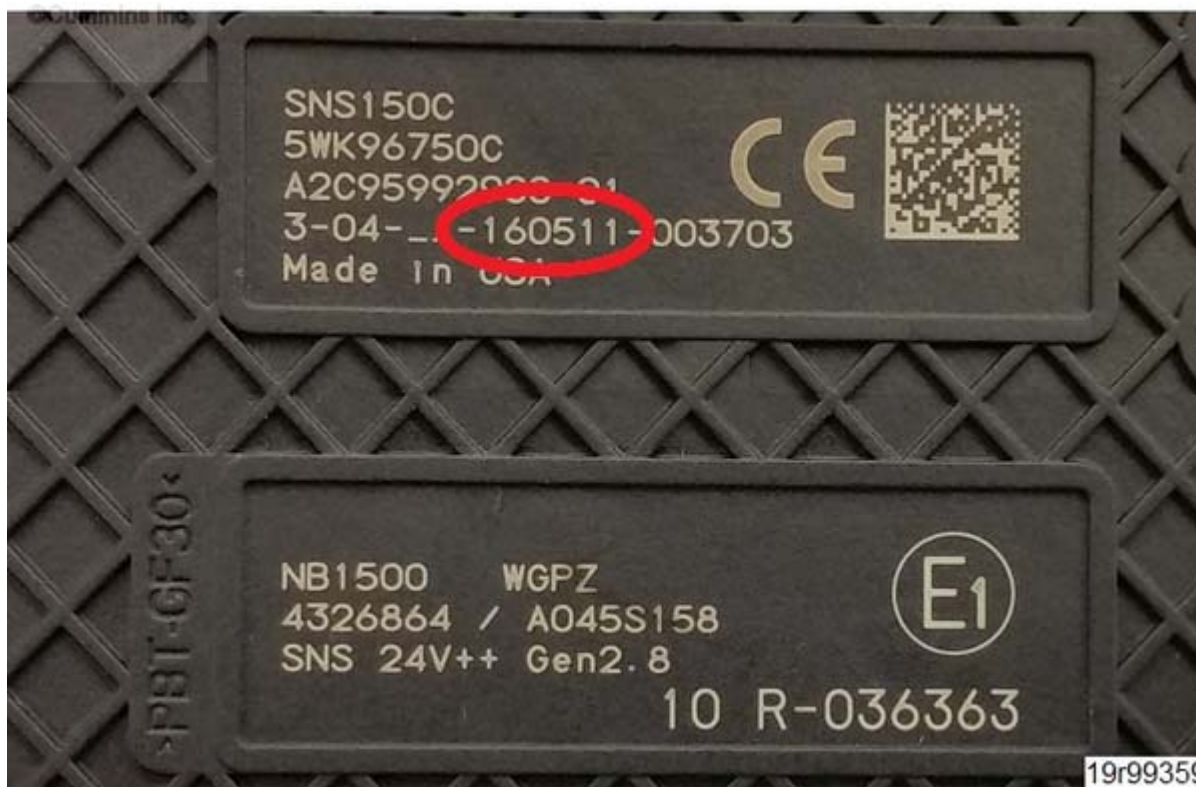
Figure 1, Aftertreatment Intake NOx Sensor Base Plate with Build Date (YYMMDD) Highlighted.
