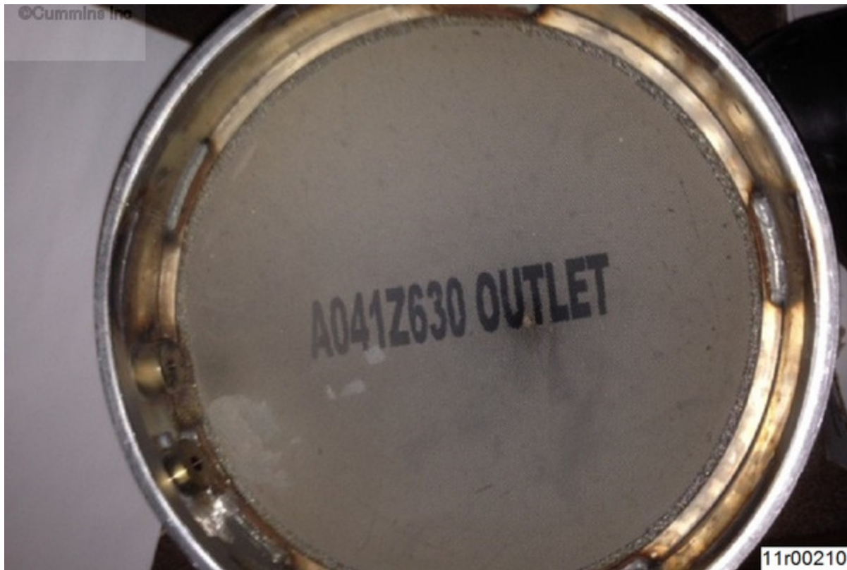
Figure 1, Previous Aftertreatment Diesel Particulate Filter Design (DPF) with Retention Ring
