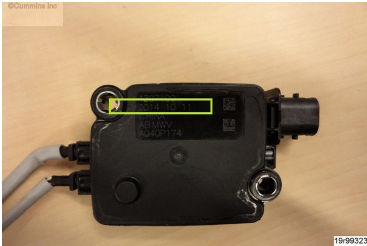
Figure 1, Date Code Location on the Aftertreatment Exhaust Gas Temperature Sensor
