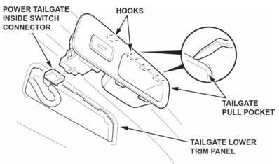
4. Pull out the tailgate lower trim panel by hand to detach the clips, then remove it.
