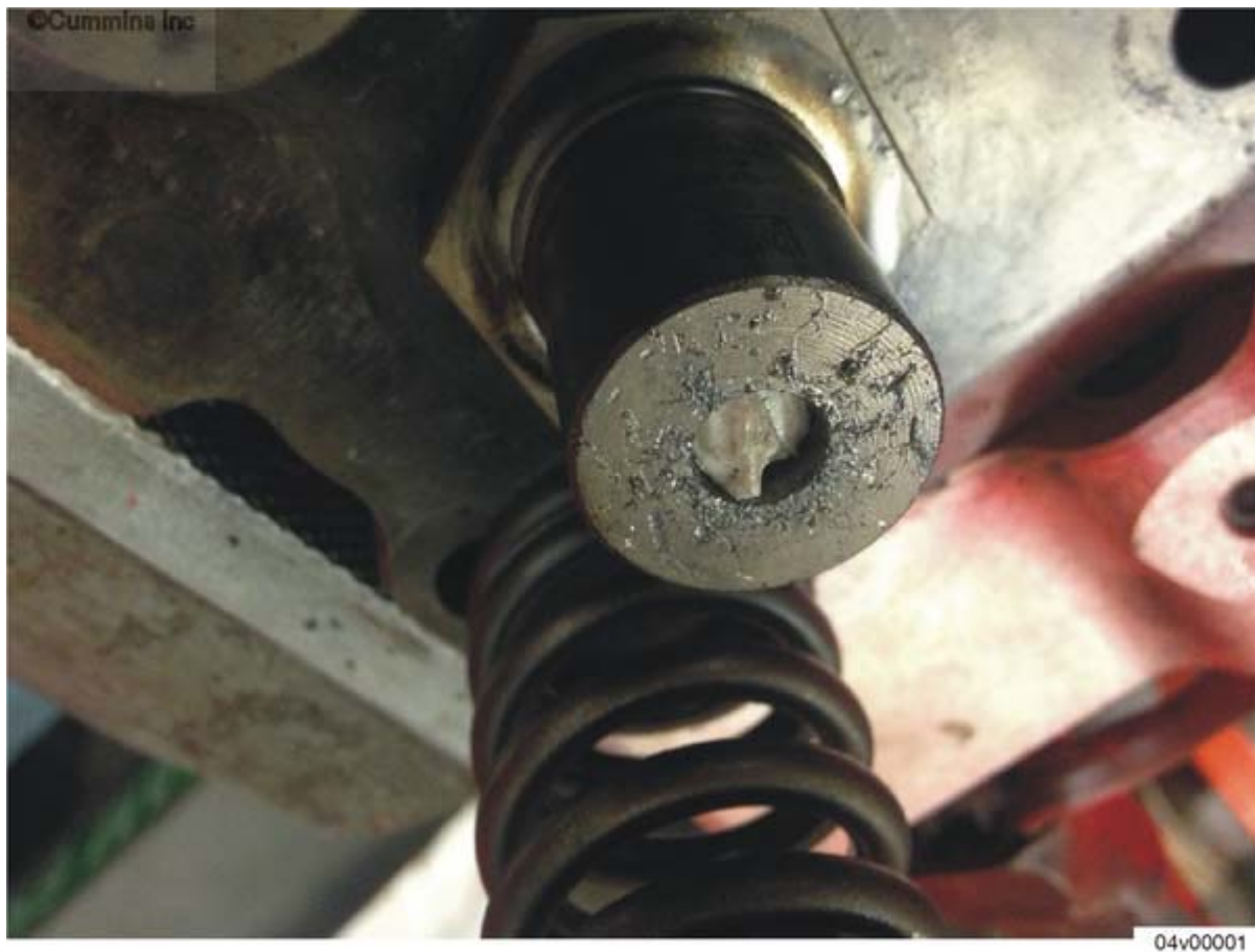
Figure 1, Fractured Fuel Pump Ceramic Pumping Plunger.
