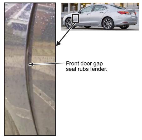
2. Open the front door on the side making the noise, and remove all of the fasteners on the front door gap seal.
