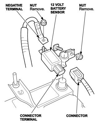
3. Remove the 12-volt battery sensor from the 12-volt battery.
